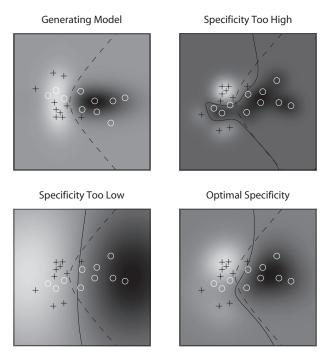
Figure 6. A two-class problem. Samples from two classes (crosses and circles) are generated from two overlapping normal distributions. In the upper left panel, the differences between the distribution densities are shown as gray levels, and the optimal decision boundary is shown as a dashed line. The other panels show kernel density estimates of the two classes with varying specificity of a Gaussian kernel, as well as the corresponding decision boundaries (solid lines).
